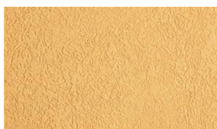
Rustic texture produced with Ceresit CT 64 acrylic plaster, grain size 2.0 mm, obtained by circular floating with a plastic float
