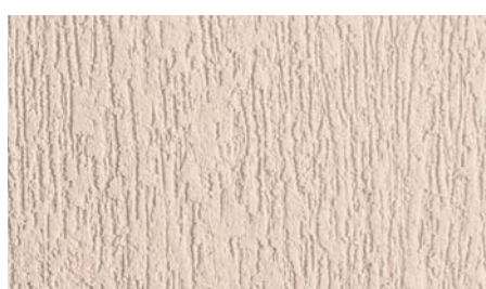
Rustic texture produced with Ceresit CT 35 mineral plaster, grain size 2.5 mm, obtained by floating with a plastic float in one direction
