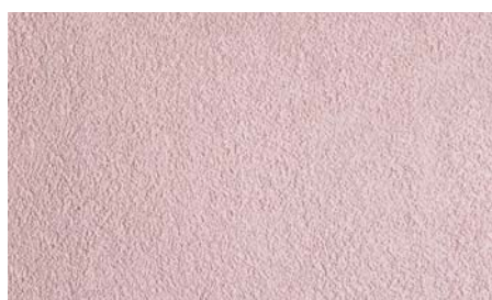
Stone texture produced with Ceresit CT 60 acrylic plaster, grain size 1.5 mm, obtained by floating with a plastic float
