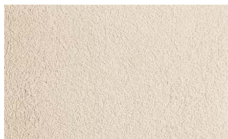
Stone texture produced with Ceresit CT 137 mineral plaster, grain size 1.5 mm, obtained by floating with a plastic float
