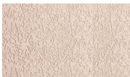
Rustic texture produced with Ceresit CT 35 mineral plaster, grain size 2.5 mm, obtained by circular floating with a plastic float
