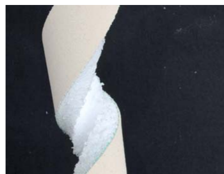
CT 100 sample: high resistance to mechanical forces
