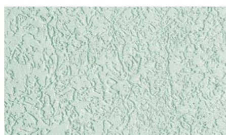
Rustic texture produced with Ceresit CT 35 mineral plaster, grain size 3.5 mm, obtained by circular floating with a plastic float
