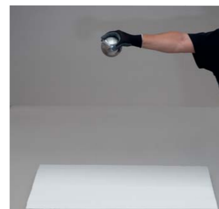
Mechanical resistance is well illustrated in the test of striking the system surface with a 5 kg ball from a height of 2 m
