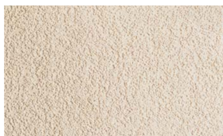
Stone texture produced with Ceresit CT 137 mineral plaster, grain size 2.5 mm, obtained by floating with a plastic float
