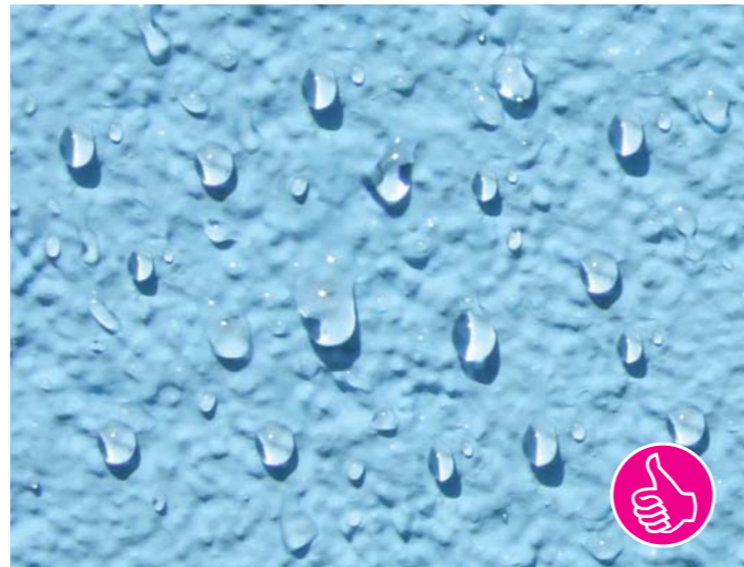
water does not soak into the structure of the paint
